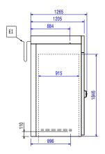
Drain ΕI Electrical inlet (power)
